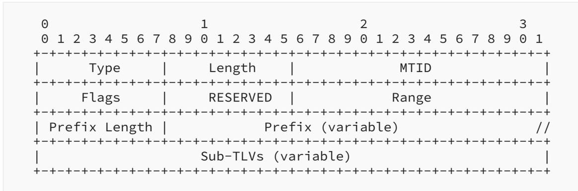
Figure 2: Multi-Topology SID/Label Binding TLV format
