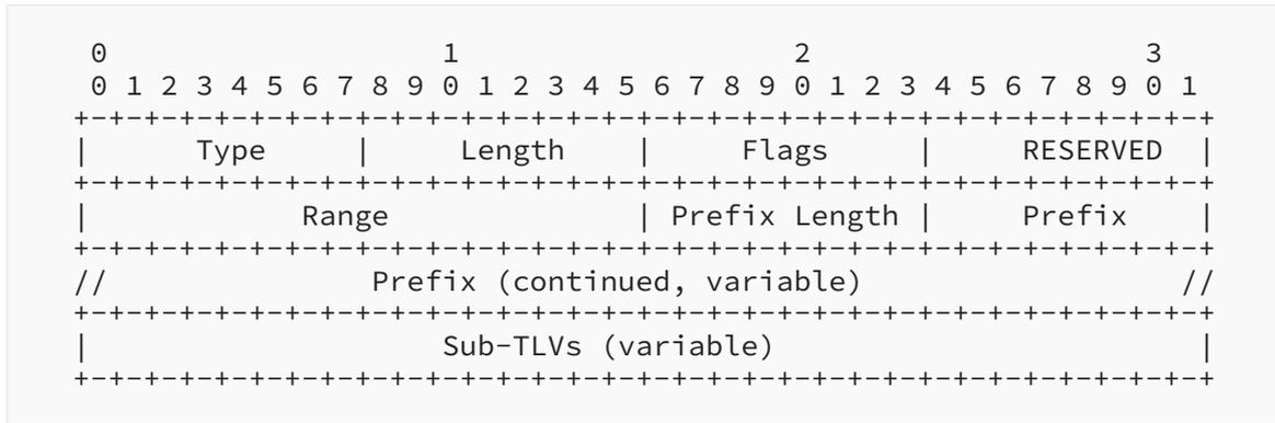
Figure 1: SID/Label Binding TLV Format
