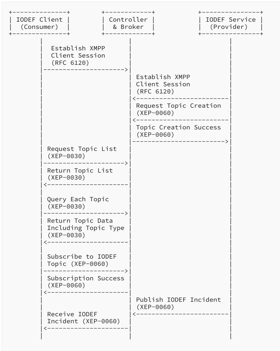
Figure 2: IODEF Example Workflow
